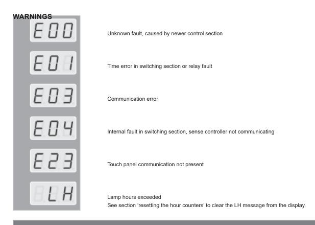
**Note:** When one of the above-mentioned fault messages appears on the display, you should no longer use the tanning appliance and the unit should be disconnected from the power. Contact ProSun for further instrcutions. (This does not apply to the LH message.)
